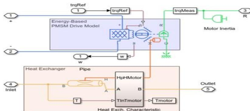
Figure 1. Electric motor.
