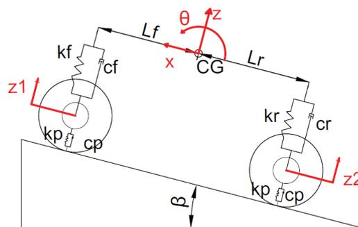
**Figure 3.** Scheme of the dynamical model.
